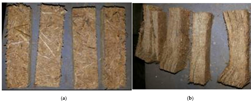
Figure 5. Compressive strength test samples—(a) before the test, (b) after the test.
