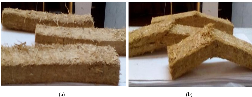
Figure 3. Samples for static bending test—(a) before the test, (b) after the test.
