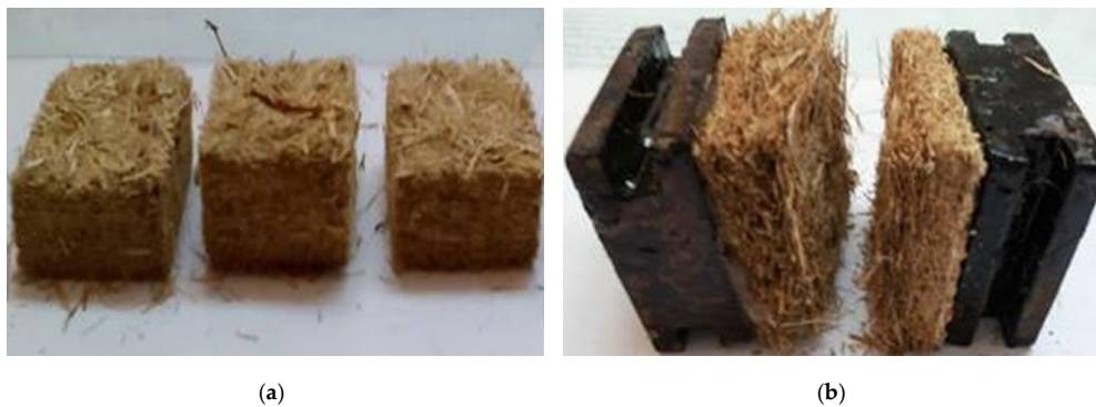
Figure 4. Samples for tension test—(a) before the test, (b) after the test.
